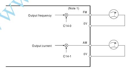
(Note 1) The maximum output voltage of the FM and AM outputs is approx. 11V.
