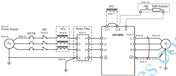
b) From U2KN11K0S, and U2KX11K0S to U2KX37K0S. For DC Drives (main aption. "), check Chapter 7-2.
