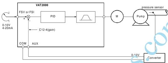
**Example of PID control configuration**
