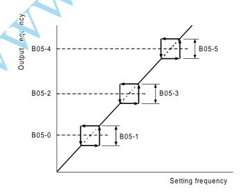
**(Note)** This function controls the frequency setting, so the above skip frequency area will be passed with a ramp function.
