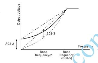
(Note) When both A02-2 and A02-3 are set, the voltage will be added as shown above.
