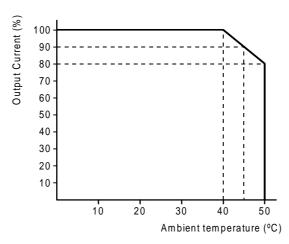
Fig. 1-1 Derating according to ambient temperatu
