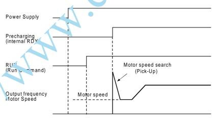
For V/f control, sensorless control C30-0=1,2,3
