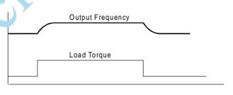
(Note 1) e slip compensation will not function in respect to the regenerative torque.
