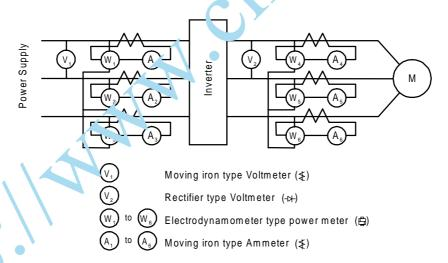
Fig. 8-1 Measurement circuit example
