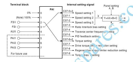
(Note) The torque setting is 300% when C07-6 is 7
