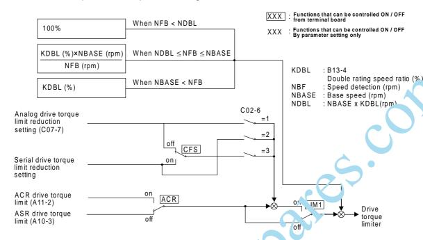
Fig. 5-12 Drive torque limit setting section
